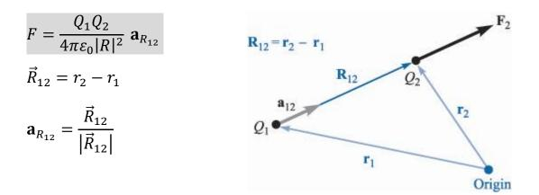
If  $Q_1$  located at ( $x_0$ ,  $y_0$ ,  $z_0$ ) and  $Q_2$  at ( $x_1$ ,  $y_1$ ,  $z_1$ ), then
